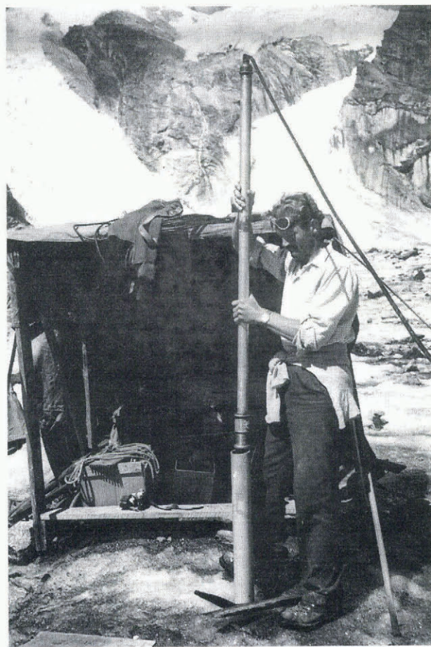
Fig. 5. The pipe in the middle section of the glacier. It became filled with ice, through leakage of water, which had frozen by pressure release, and Bill Ward is here inserting a heated element to melt it out.
