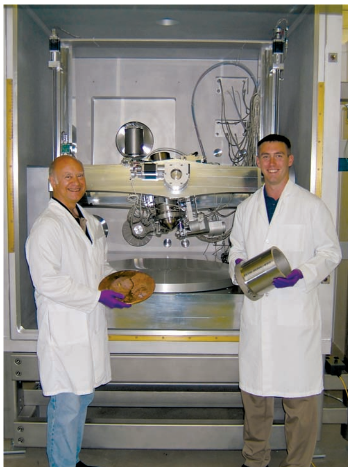
Figure 1: A large chamber scanning electron microscope (LCSEM) used by the Y-12 group of the Oak ridge National Research Laboratory
