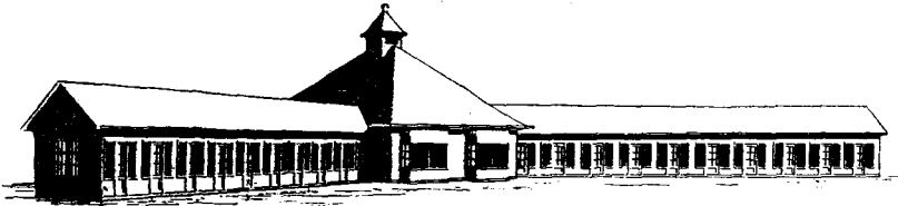
Fig. 29. Elevation of part of a sanatorium pavilion of Doecker construction for 20 beds. The administration buildings are not shown
