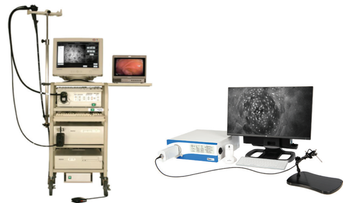
Figure 4: First- and second-generation devices from Optiscan. Left. Pentax ISC-1000 integrated with Optiscan's confocal scanner. Right. Optiscan's second-generation laboratory device, FIVE2 (ViewnVivo).
