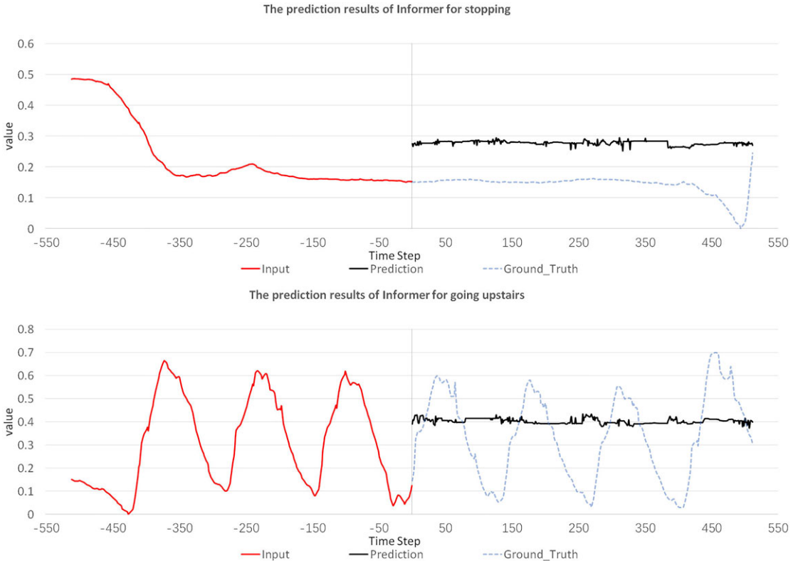
Figure 6. Predicted trajectories of the Informer model for different gait types. The value of the y-axis in the picture represents the value of the normalized gait angle.
