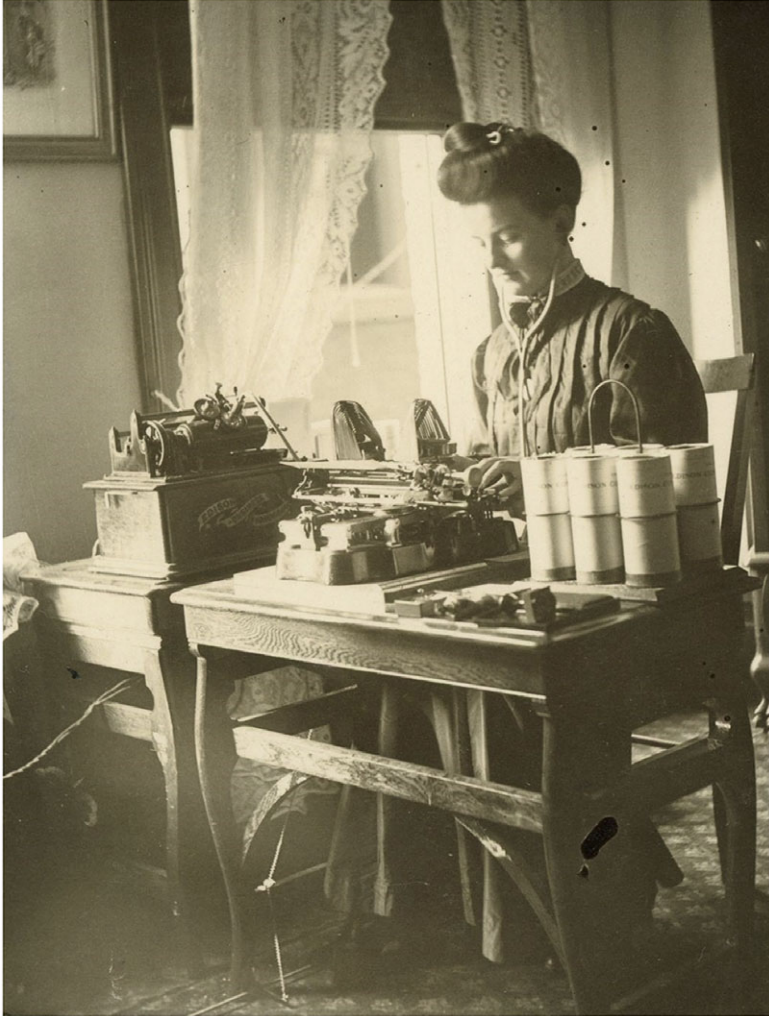
Figure 17. Miss Brady listening to Edison dictation machine and transcribing on Oliver typewriter, Philadelphia, 1905, Thomas Edison National Historical Park, U.S. National Park Service, West Orange, New Jersey.
