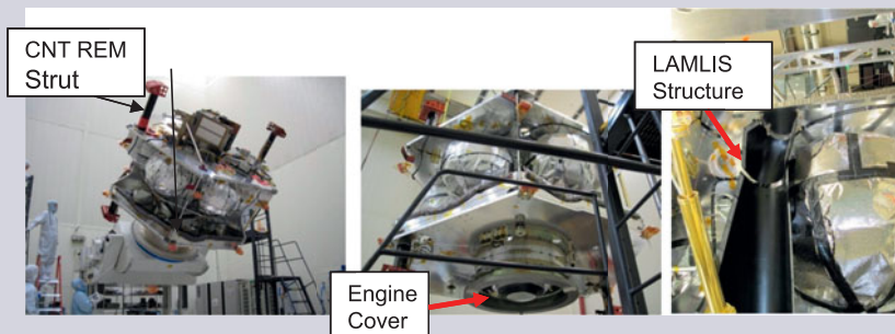
Figure 1. Carbon nanotube- (CNT)- based composite rocket engine motor (REM) struts and engine cover panel and carbon nanostructure-based composite linear actuator multilayer insulation support (LAMLIS) structure incorporated in the Juno spacecraft inherently provide electrostatic dissipation protection.
