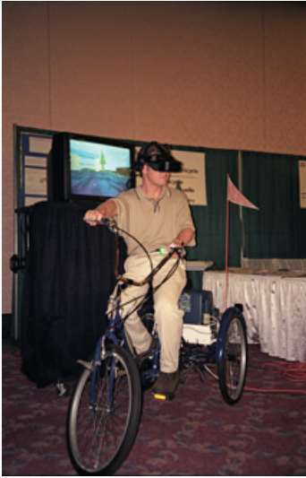
Figure 17 Aligning the virtual visual and physical worlds. (a) This part shows the VR trike. Trike motion is monitored by wheel and handlebar encoders enabling an individual to cycle around an extended visual world as head tracking is performed relative to the trike. (b) This part shows one of the authors wearing Apple’s Vision Pro which can be worn while walking around a real environment.
