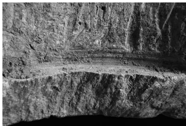
Figure 12. Detail of the rough interior of the fragmented vessel: trace left by a large rotating gouge.
