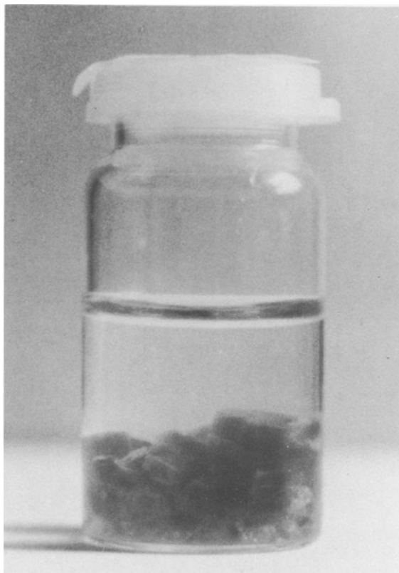
Figure 3. Photograph of a typical sample after swelling for two weeks. The height of the sample jar is approximately 5 cm.
