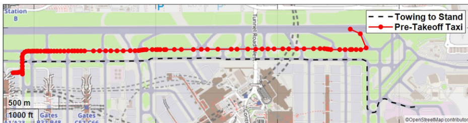
Figure 23. Example of towing trajectory prior to pre-takeoff taxi. ADS-B data from Flightradar24 [24]. Map data from OpenStreetMap ( https://www.openstreetmap.org/copyright ).
