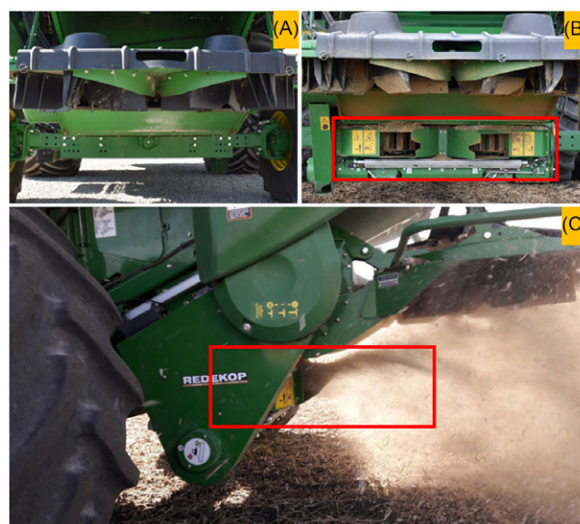
Figure 1. The Redekop™ Seed Control Unit/seed impact mill (a harvest weed seed control method) installed on a John Deere S680 combine in 2021 on a commercial farm in Gilbert, IA. The figure shows the rear of the combine without seed impact mill (A); impact mill installed to the combine (B); weed seed-bearing chaff exiting through the impact mill (C).
