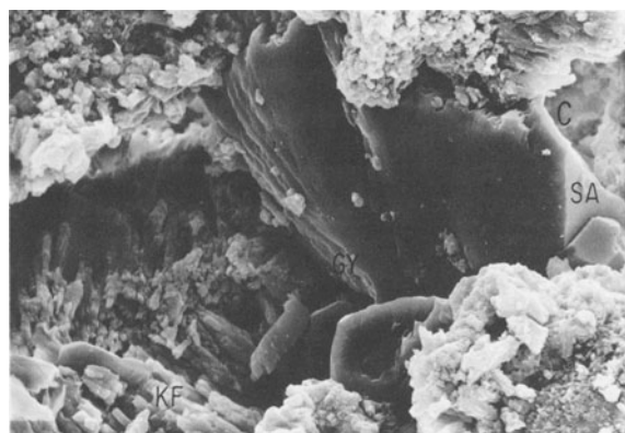
Figure 5. Scanning electron micrograph of altered vitric tuff showing sanidine phenocrysts (SA), K-feldspar altered from glass (KF), chalcedony (C), and gypsum (GY). Sample M10. Horizontal bar is 10 \mu\text{m} .
