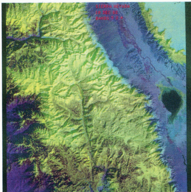
Fig.3. Thematic Mapper image of the southern Sierra Nevada. Blue = TM2, green = TM4, and red = TM3. The dimensions of the scene are 85 km × 80 km. It is sub-sampled such that only every sixth pixel is printed, because the size of our image display screen is 512 × 512.
