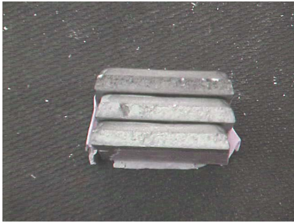
Fig. 1 Fracture surface of the piece with the defect.
