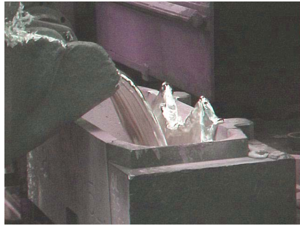
Fig. 2. Liquid cascading into the mould
