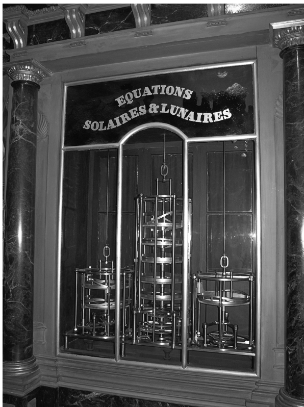
Figure 3.2 The Strasbourg Astronomical Clock contains three mechanical integrators for summing Fourier series that calculate the positions of the sun and the moon. The series is summed mechanically by using cams riding on cams. The cams have a cosine wave profile that repeats once, twice, three or more times per revolution. The size of the profile determines the strength of contribution to the summation. The left integrator has two terms in the series, the centre six terms and the right integrator just one. (From Wikipedia; photo by David Iliff. Licence: CC-BY-SA 3.0)
