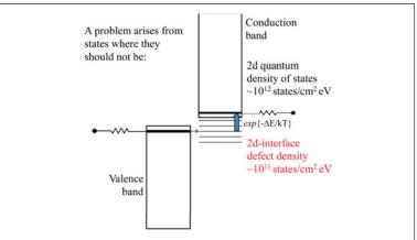
Figure 2. Tunneling-assisted current generation from shallow traps has emerged as one of the major undesired leakage mechanisms in tunnel field-effect transistors. This is a two-step process, tunneling followed by thermal activation. It produces a leakage current that prevents sharp switching.
