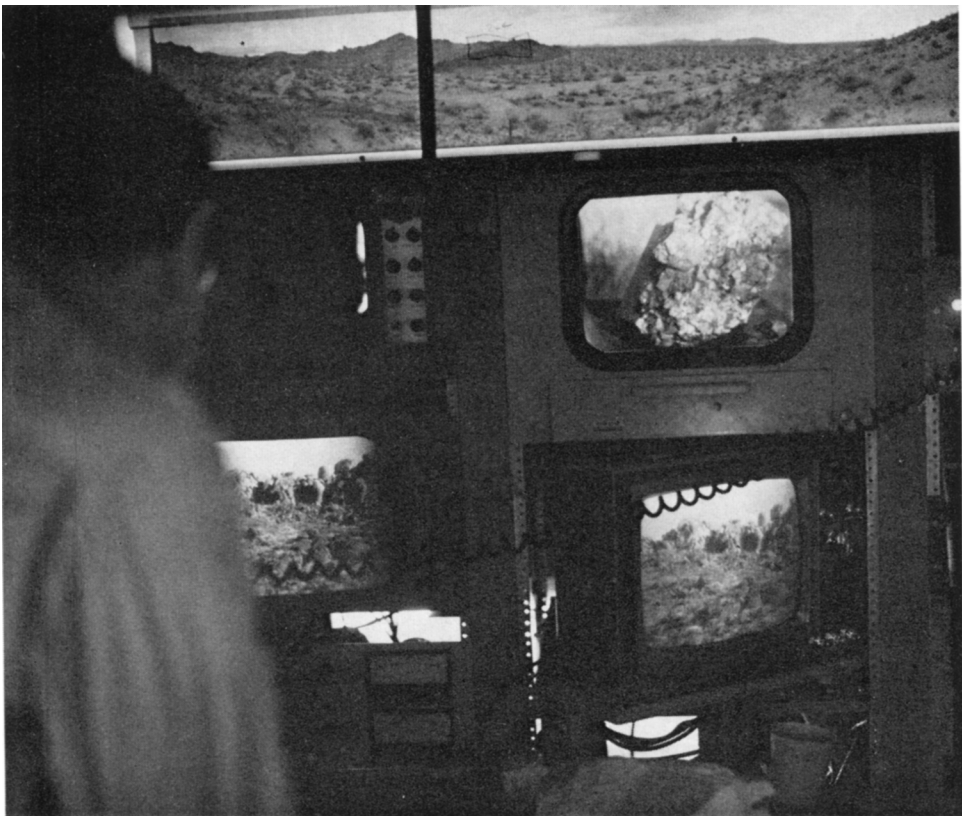
Fig. 7. Visual displays inside field-test truck. Top: panorama, simulating photofacsimile display. Center: TV close-up of rock sample. Bottom: two views of local scene.
