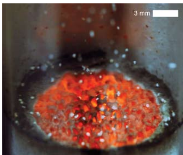
Figure 6. Front face of a catalyst during reforming of approximately 230- \mu\text{m} particles of cellulose in air. 11
