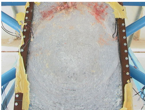
Figure 15. Windshield after bird impact test.
