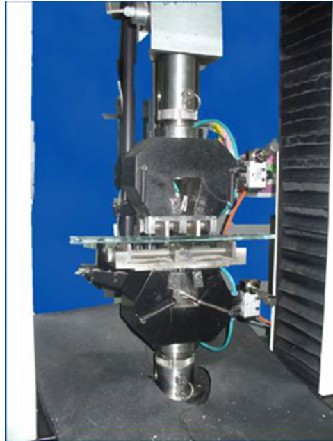
Figure 5. The three-point bending test device.
