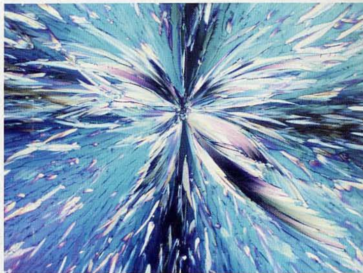
Figure 2. TNT recrystallized spontaneously from a supercooled (to room temperature) melt, crossed polars, 80X.
