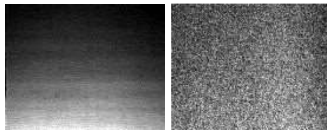
Figure 4. The spatial distribution of the intensity of the fundamental using the [Ru,B 4 C] strip, detuning the second crystal of the MLM (left, averaged over the energy range 11.5-12.4 keV) and the first harmonic (right, averaged over the energy range 22.8-23.4 keV).
