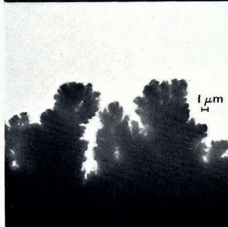
Fig. 3. (a) Hexagonal ice crystals grown on a copper grid at -110^{\circ}\text{C} , (b) electron diffraction pattern of (a) showing prominent spots and faint rings, (c) hexagonal crystals grown further in the direction of the electron beam, (d) the characteristic needle-like patterns of the electron diffraction of (c)
