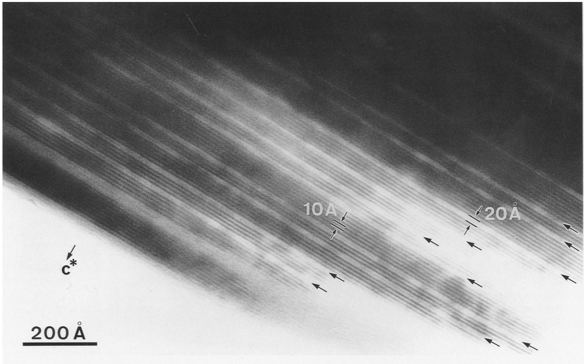
Figure 6. Lattice fringe image illustrating sporadic distribution of single vermiculite layer ( \downarrow ) after 1 day of reaction at 80°C in the 20 ml experiments.
