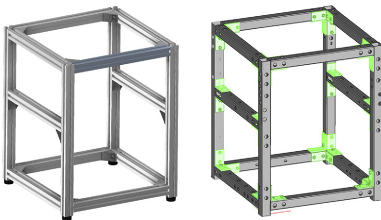
Figure 3. Left – Original aluminum profile frame. Right – Modified steel SHS frame with brackets.
