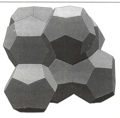
Arrangement of the cells that make up the new minimal structure reported by Weaire and Phelan. It consists of six 14-sided polyhedra and two 12-sided polyhedra. This is the repeating unit on a simple cubic lattice.
