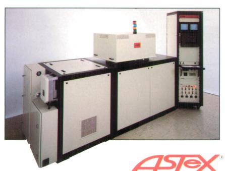
The all *new* LADS represents a significant advance in New Diamond technology. Using a rapidly flowing reactant stream, LADS will produce *high quality* diamond films over large areas and complex contours. ASTeX is prepared to provide processing support for special applications and help develop fixtures for odd shaped items.
