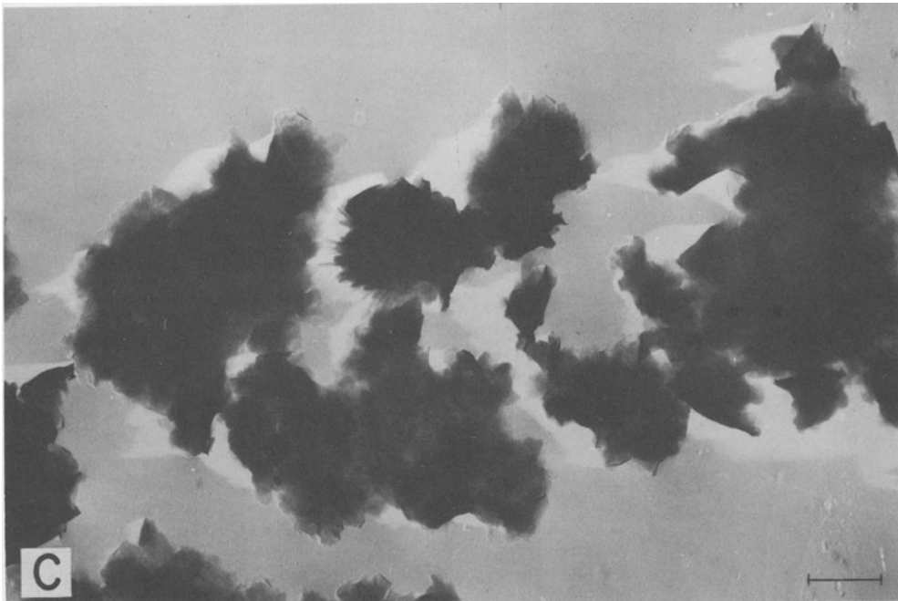
Fig. 4. Electron micrographs of equilibrated Belle Fourche montmorillonite samples. A has crystalline kaolinite added initially. B formed no kaolinite. C formed considerable kaolinite. The line indicates 1\ \mu in all photos.
