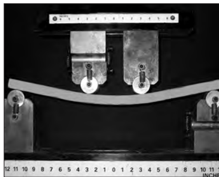
Figure 1. Bendable engineered cementitious composites (ECCs) subjected to flexural loading. The beam specimen measures 304.8 mm long by 76.2 mm wide by 12.2 mm deep; deflection is 22 mm at a peak load of 0.6 kN. The maximum tensile strain capacity shown here reaches 3–5%.
