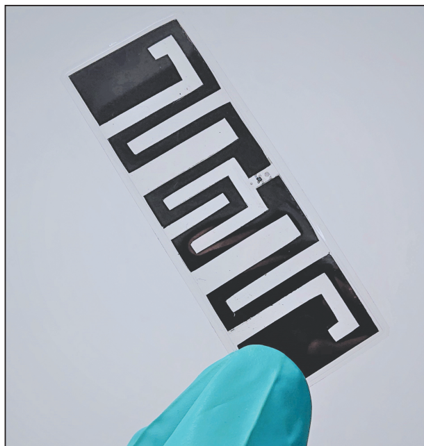
Nanotech graphene inks could print eco-friendly RF tags that cut waste. Credit: University of Sussex.
