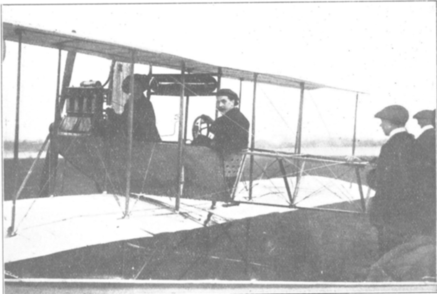
Fig. 2.—The original Avro Tractor Biplane, built in 1911. Fitted with 35 h.p. Green Engine. This machine was the first Tractor Biplane ever built.
