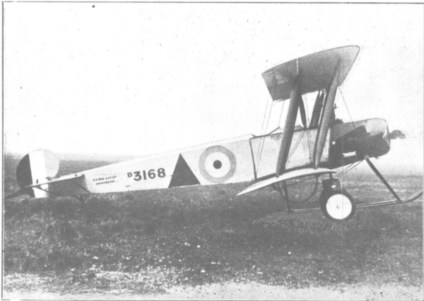
Fig. 14.—Avro Type 504 J. Engine, 100 h.p. Monosoupape Gnôme. A machine belonging to the School of Special Flying at Gosport.
