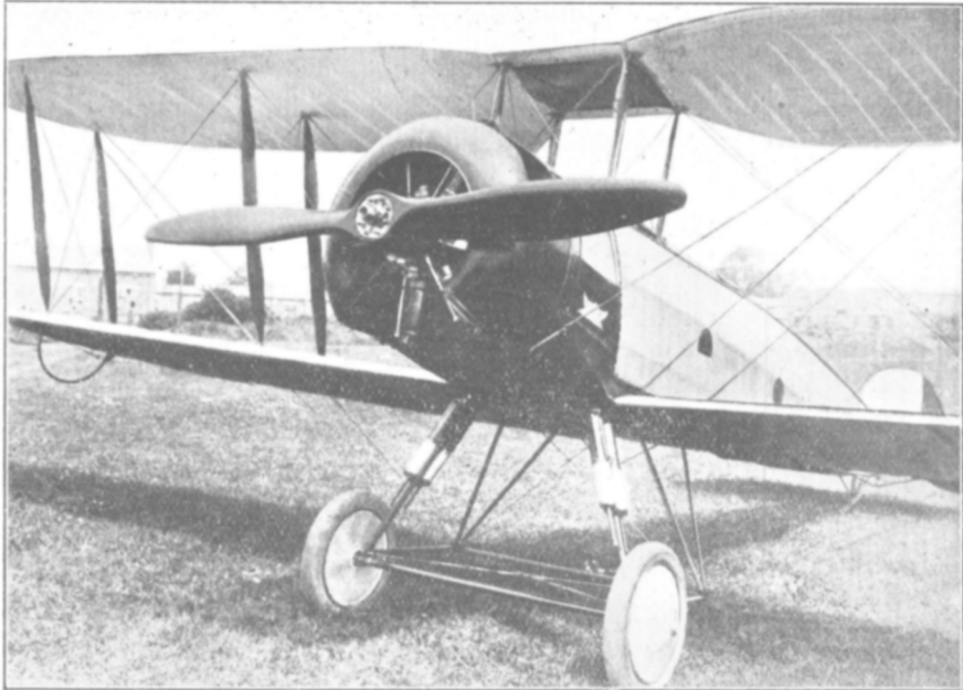
Fig. 30.—The latest edition of the Standard Training Machine, showing new Oleo Undercarriage and cut aways at wing-roots and centre section, to improve visibility from front cockpit.
