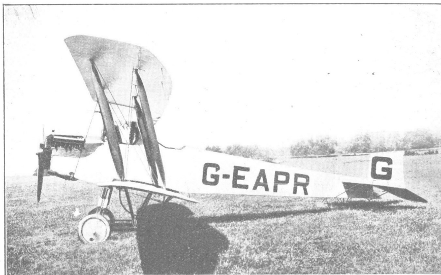
Fig. 23.—An Avro 504 fitted with 180 h.p. Wolseley "Viper" Engine.
