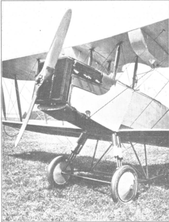
Fig. 24.—A close-up view, showing the installation of the "Viper" Engine.
