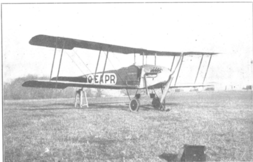
Fig. 15.—An Avro 504 Type, fitted with a 90 h.p. Curtiss Engine.
