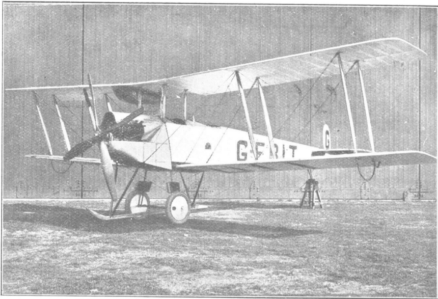
Fig. 19.—An Avro fitted with an 80 h.p. Renault Engine.
