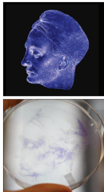
Figure 7. Light is used to induce cells to produce a biomaterial, specifically a functionalized bacterial amyloid fiber. With optogenetics, remarkable resolution and control of this biomaterial are achieved. The top pattern is the light mask (an extrapolation of a da Vinci sketch) that is shone on a liquid culture of engineered E. coli , and the bottom is the resulting biomaterial produced by the cells and then stained with crystal violet dye on a petri dish. Credit: Christopher Voigt and Felix Moser, Massachusetts Institute of Technology.
