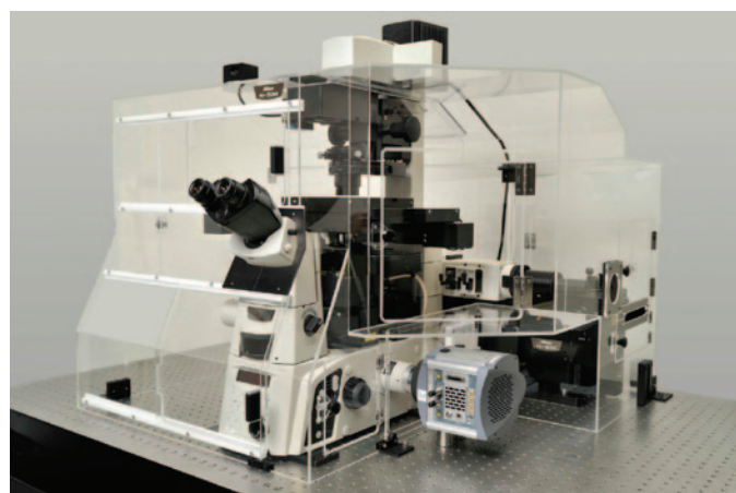
Figure 1: The N-SIM super-resolution microscopy system built around a Nikon Ti-E inverted microscope.
