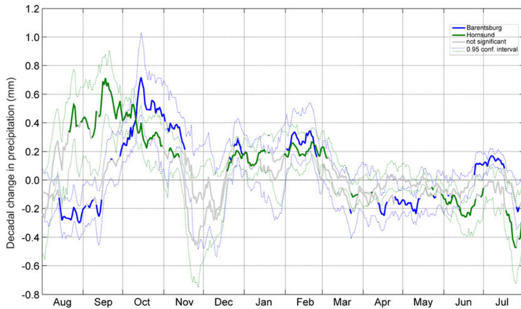
Fig. 13. Comparison of the estimated trends in daily total precipitation (change per decade) at Barentsburg and Hornsund meteorological stations for the period 1 August 1984–31 July 2016. The results were obtained for the MASH-filtered data.
