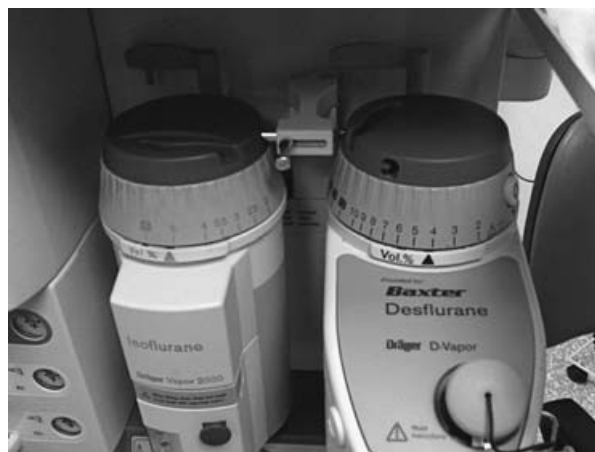
Figure 2. Isoflurane vaporizer at 5% with interlocking device on and desflurane also switched on at 4%.
