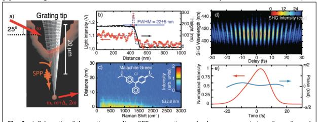
**Fig. 2.** a) Schematic of the grating-coupling, SPP propagation, and subsequent re-emission of nanofocused excitation. b) Spatial extent of the nanofocused excitation. c) Grating-coupled TERS of a monolayer of Malachite Green on an Au surface. d) FROG measurement acquired with SHG generated at the tip-apex by nanofocused SPPs, demonstrating a pulse duration of 16 fs as determined by e) FROG reconstruction of the temporal profile and phase of the pulse.
