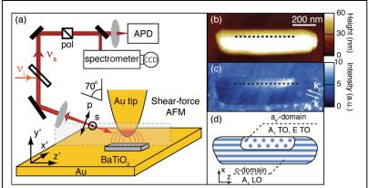
**Fig. 1.** a) Experimental TERS setup to allow for optical nanocrystallography. b) Shear-force AFM topography and c) corresponding spectrally integrated TERS signal showing a ferroelectric domain as illustrated in d).
