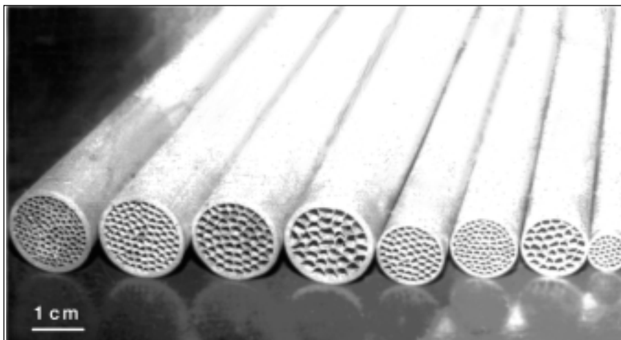
Multichannel tubes produced by the multichannel porous materials (MPM) technique.
