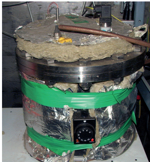
FIG. 1. Container prepared for Magnox swarf corrosion monitored (hydrogen gas pressure increase technique).
