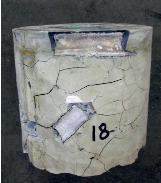
FIG. 6. A 3 l product at 7.2 wt.% Magnox corroded.
