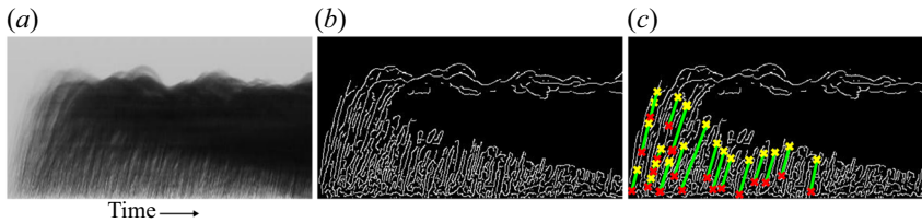
Figure 13. Procedure used to estimate the speed of the rising fountain flow in our experiments. (a) Grey scale centreline time series showing rising fountain mixture (forward-sloping lines), (b) output of the edge detection function in Matlab and (c) output of Hough transform used to calculate the gradient of the forward-sloping lines in the time series.
