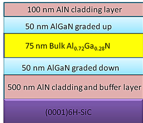
Figure 20. Schematic representation of the investigated GRINSCH double heterostructure. [134]
