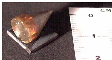
Figure 1. Example of AlN boule grown at Crystal IS.
