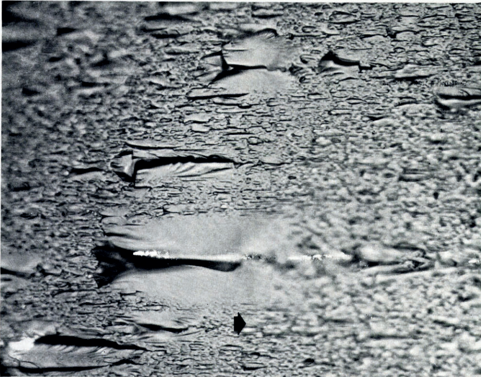
Fig. 6. Two types of mist zone features. Arrows show direction of crack propagation. (Photograph from Johnson and Holloway (1968).)
