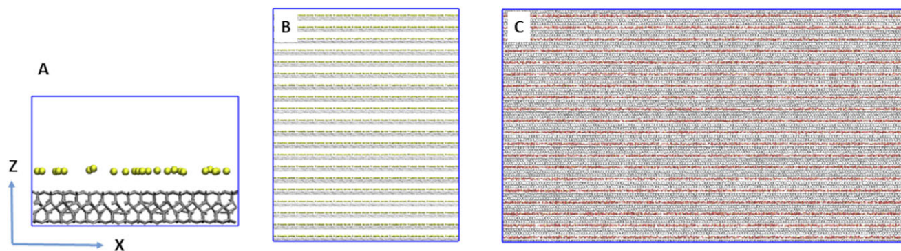
Figure 2. Model preparation for large-scale MD simulation of Na-Mnt with heterogeneous interlayers. (A) Initial simulation box with one clay layer (gray) and Na + ions (yellow). (B) Large clay structure by replicating clay structure in A. (C) Homogeneous 1W configuration (water O red) with dimensions ~ 41.6×7.1×23.3 nm 3 .
