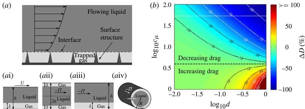
FIGURE 1. (a) Schematics of laminar flow over an idealized superhydrophobic surface, with four flow configurations considered: (ai) Couette flow; (a(ii)) symmetric pressure-driven channel flow; (a(iii)) one-sided pressure-driven channel flow; and (a(iv)) pipe flow. (b) Change in drag,  $\Delta D$ , as a function of viscosity ratio ( $c_\mu$ ) and lubricant thickness ( $d$ ), for a laminar Couette flow configuration (ai) with no net mass flow in the lubricant layer (from Busse *et al.* 2013).
