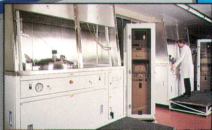
Production UHV for heat treatment
