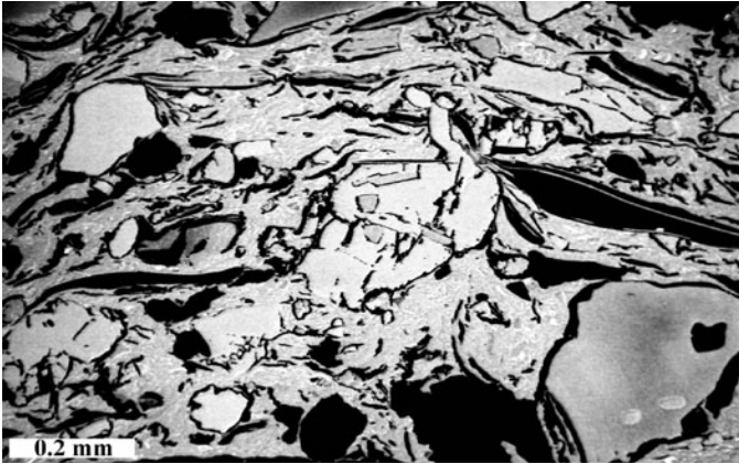
Figure 7: Higher magnification view of the microstructure of a pottery shard. Note that the clay microstructure consists of two phases that may be the result of incomplete transformation to mullite.
