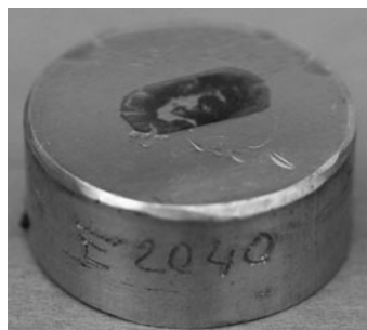
Figure 2: Photograph of a 1-inch diameter Cerrotru alloy mount of a partially reduced Taconite (Hematite) pellet from Shultz et al. [5].
