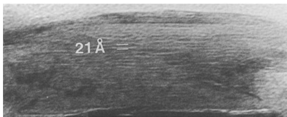
Figure 5. Lattice-fringe image of a thick lath of a 7-Å phase (of kaolinite type). Note the regular 21 Å basal spacing along c^* of this particular polytypic sequence.
