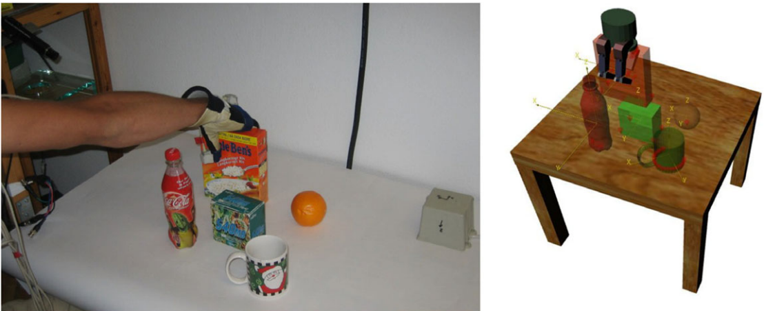
Figure 10. The robot is guided to grasp by manual demonstration. Left: The human is moving a box. The system recognizes which object has been moved and chooses an appropriate grasp. Right: The robot grasps the same object using the mapped version of the recognized grasp (the images in Fig. 10 are from ref. [61]).
