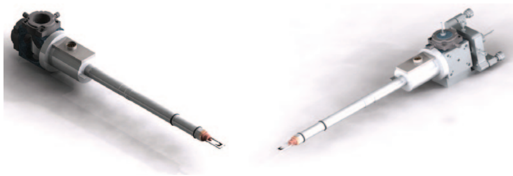
Figure 1: Two versions of the Multimodal Optical Nanoprobe system for electric biasing, scanning tunneling microscopy imaging, and light optical spectroscopy with the external aligner. For details see US patent publication US2010/0102248A1 [7].
