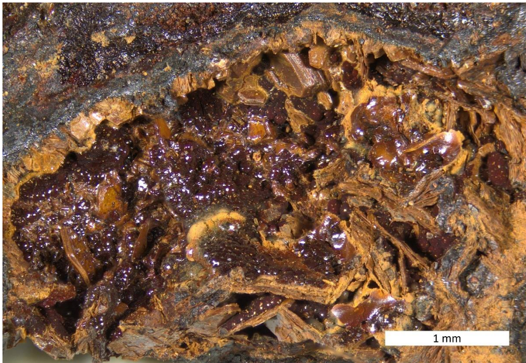
Figure 2. Colour image of a cavity with akaganeite crystals and dark brown, botryoidal goethite. Sample GEO-NRM #20040065.
